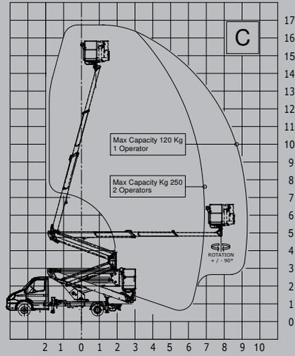
**CROSSBEAMS ONE SIDE FULLY OPENED ONE SIDE CLOSED**
