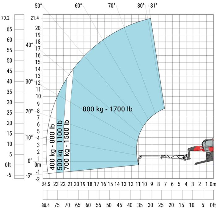
Machine on lowered stabilisers with hook 6000 kg (Metric)
